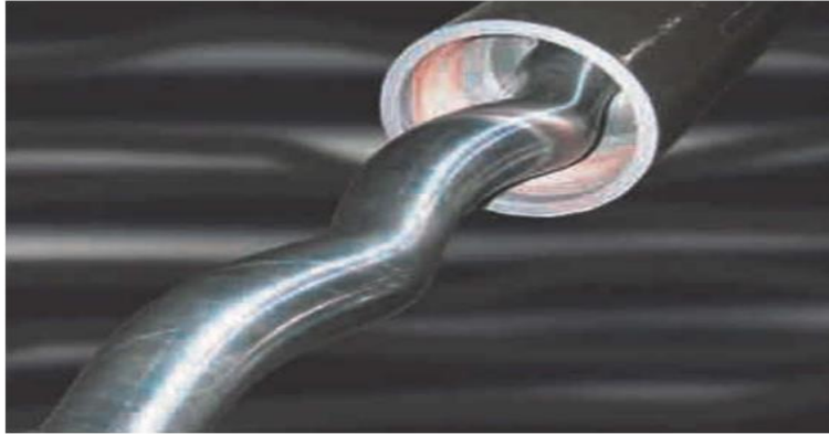
Figure 1.16 Single lobe PCP 1-2, rotor and stator view
