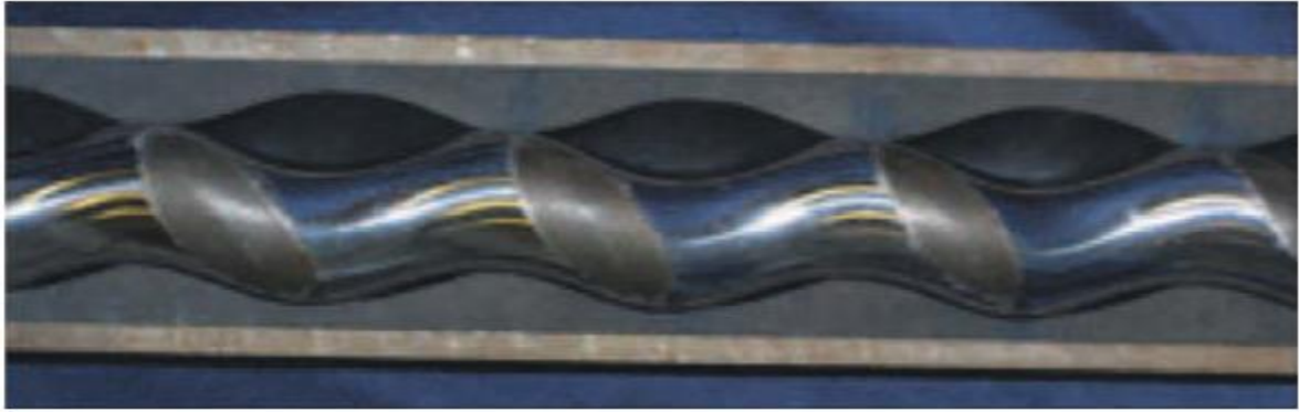
Figure 1.17 Crest of rotor wear
